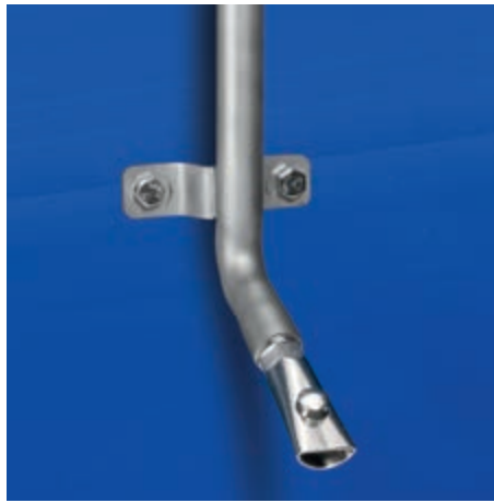
Nipple drinker with bite ball for sows and finishing pigs (high and low pressure), minimal water losses because the animals need to take the entire nipple into their mouths
